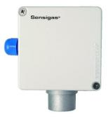
11...28Vdc power supply. Pellistor (S (standard) or P (professional) version) or Semiconductor (T version) sensing element for flammable gases; Electrochemical Cell (S or P version) or Semiconductor (T version) for toxic gases. Up to three alarm thresholds. Led on the sensing element for operating status indication. Automatic countdown of sensor lifetime.
