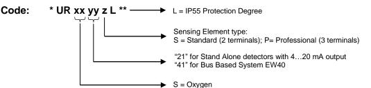
\* Prefix to the name of the Detector: DR = Display with Relays; DN = Display without Relays;
