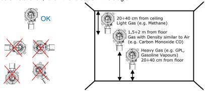
The positioning of the sensors must take into account not only the aforementioned general rules, but also the following installation rules; in particular the sensors must be installed:
