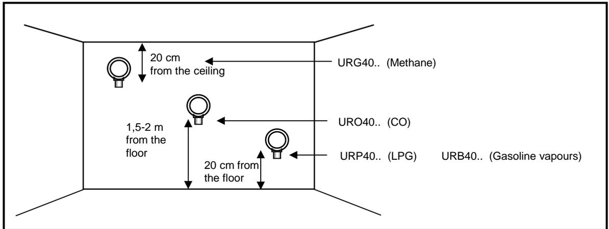
Fig. 3.4 – Possible detector positions
