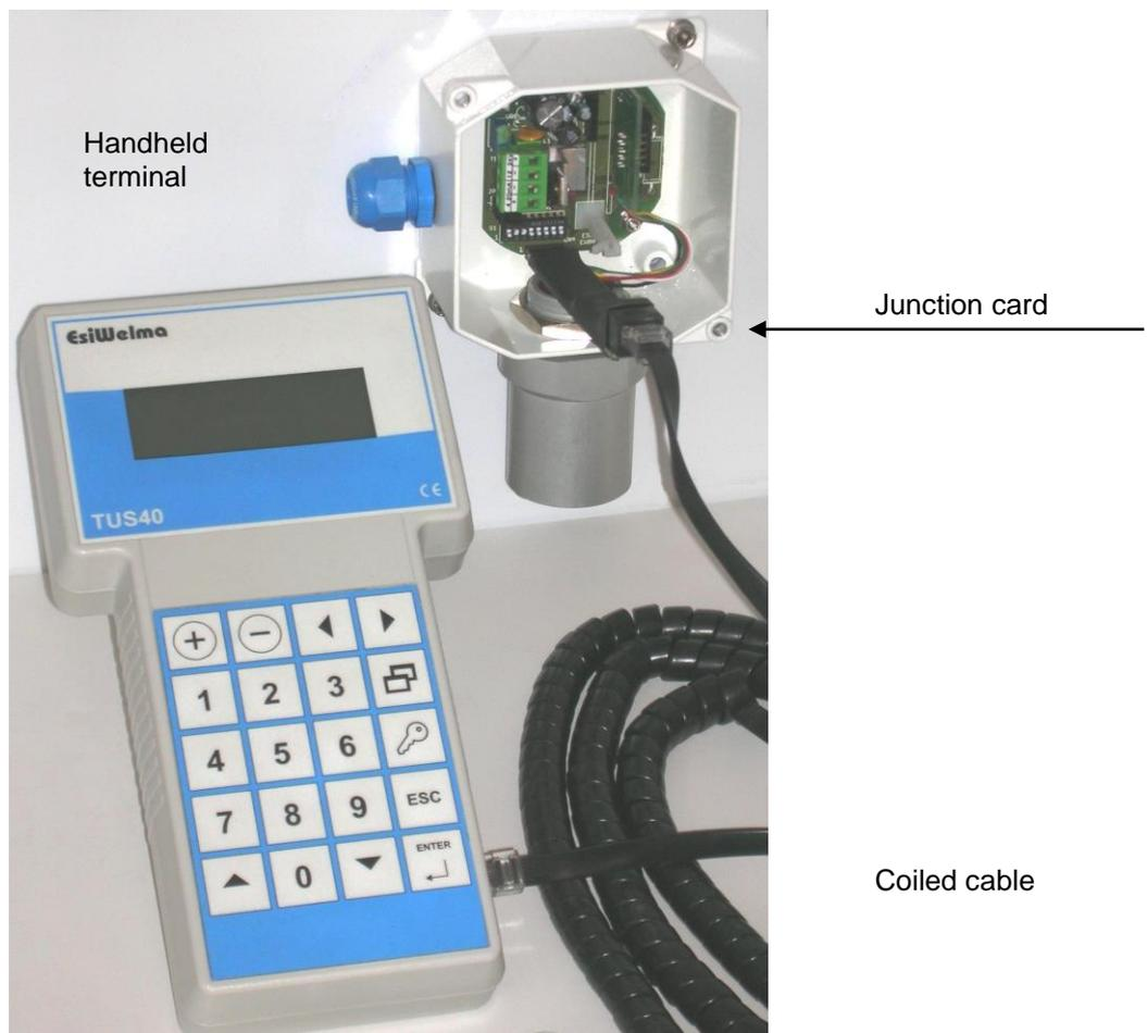
Fig. 2.1 – Terminal unit for monitoring and setting UR.20.. sensors
