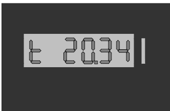
Figure 15: Example of wrong fuel distribution display
