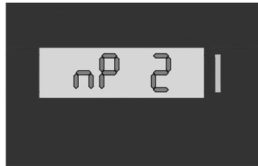
In this case the parameter allows to choose if encoder has to use 1 or 2 channels.
