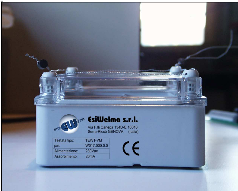
Photo 6: Computing head TEW1-VM identification plate
