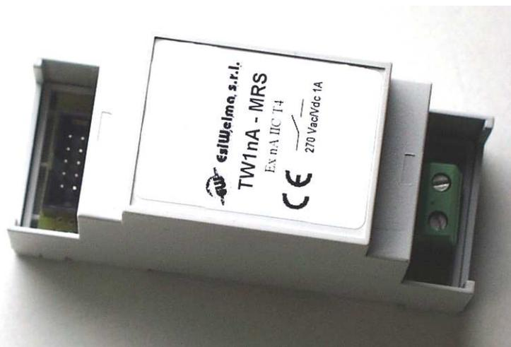
**Photo 7:** Anomaly remote signalling device
