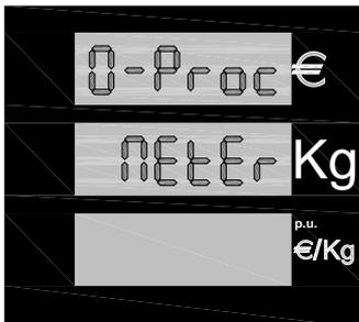
It means the procedure has to be started only after the mechanical and electrical installation of the whole dispenser on the refuelling station. The whole sequence is automatic; when it stops, parameter is set to zero and the computing head is ready to deliver. In case a black out occurs during this procedure, parameter is set to zero and operator has to start the procedure again.
