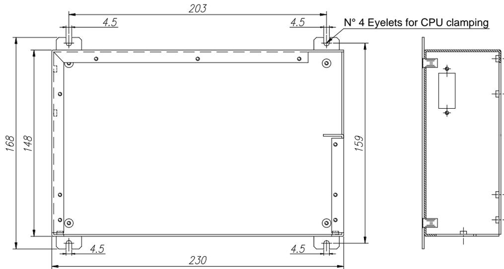
**Figure 30:** Clamping of the CPU box
