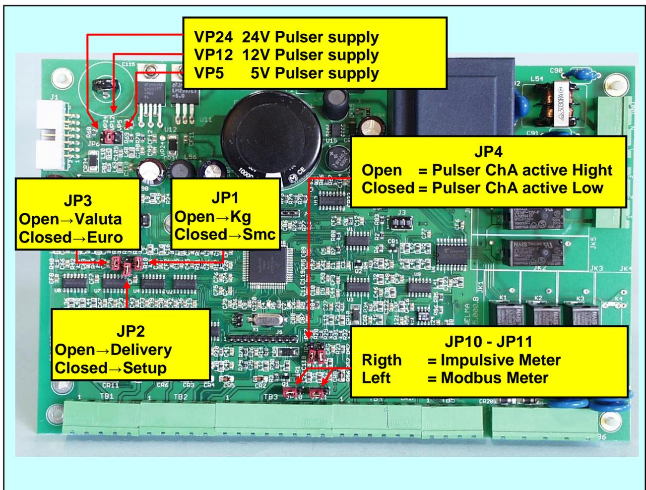
Photo 4: Set-up jumper on CPU
