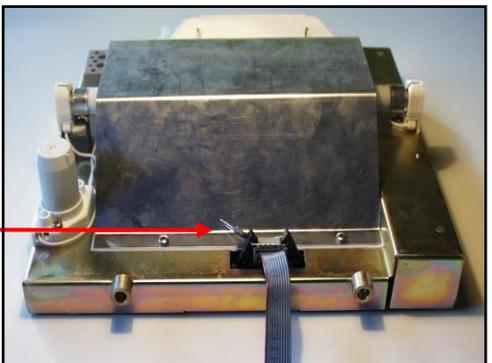
Photo 13: Computing Head TW1-M and TW1nA-M Display rear view . Neon tube back-lighting version
