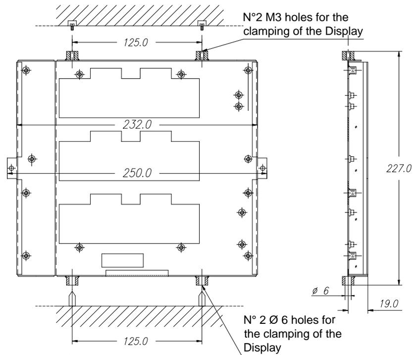
**Figure 31:** Clamping of the display box
