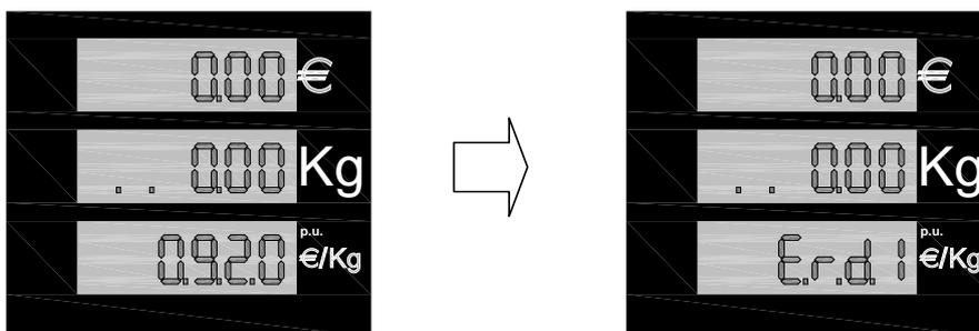
Figure 27: Passage from delivery to block during an "anomaly simulation" phase.
