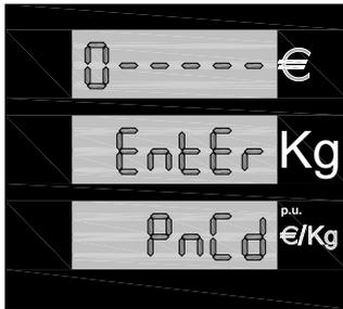
After pressing red «S» button and entering the set-up, the computing head asks for password; if it has not been previously modified, its default value is 10000. To enter the exact code, follow the procedure below:
