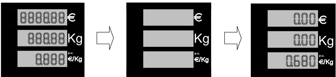
**Figure 3:** Refuelling start sequence; CNG metric counting version
