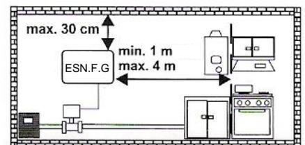
The detector **must not** be installed:
