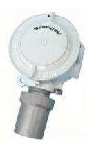
11...14Vdc power supply. Sensing element - catalytic (S version), pellistor (P version) or semiconductor (T version) for explosive gases, and electrochemical cell (S or P version) or semiconductor (T) for toxic gases. Up to three threshold limit values. LED on the sensing element for operating status indication. Automatic countdown of sensor lifetime.
