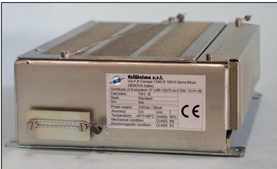
Photo 9: Identification plate on electronic computing head TW1
